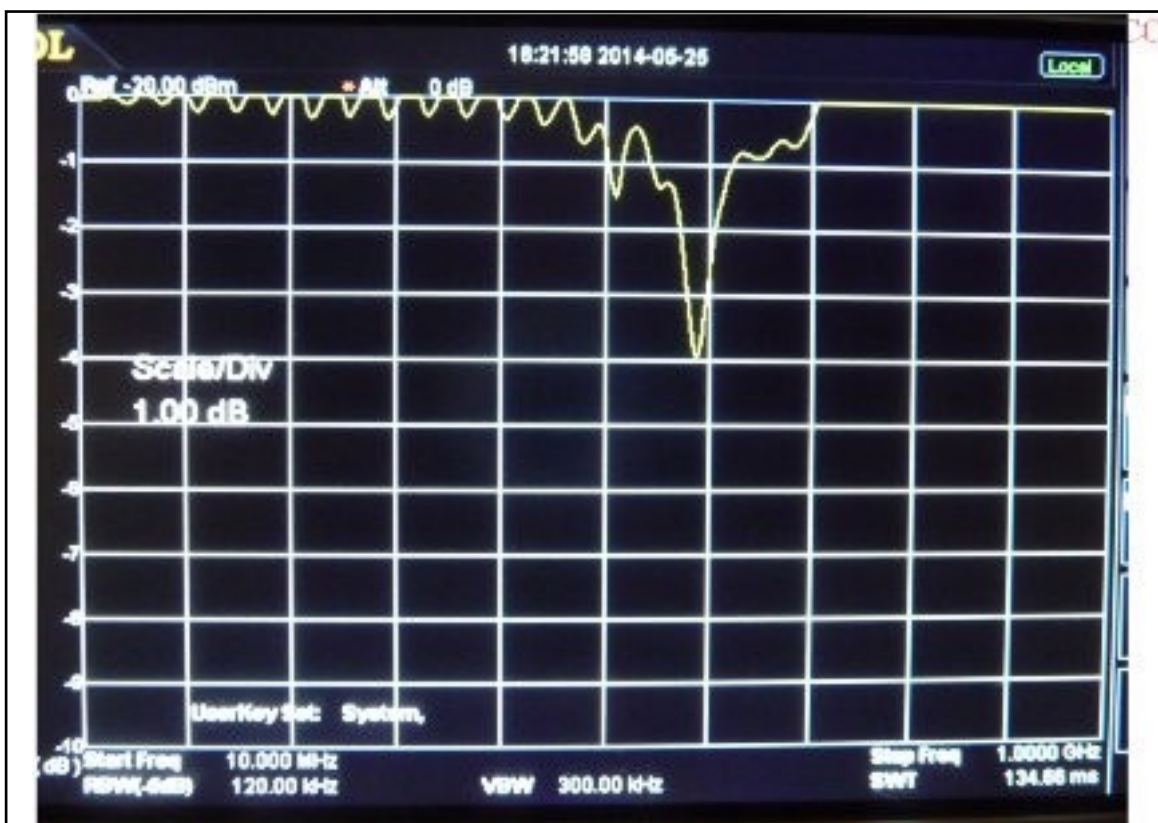
Figure 32 Looking for shielding imperfections with a reflectometer - the display (8)
